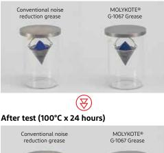
Test method: Oil bleed (JIS K 2220 100°C x 24 hours) - grease is colored for testing
