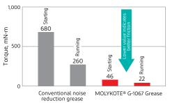
Test method: Low-temperature torque test (JIS K 2220).
